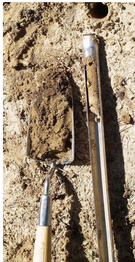
You can use a trowel or a soil auger to gather your soil samples.
