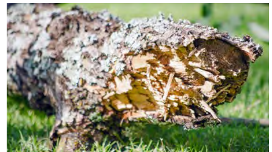
Figure 3. Police photo showing the broken end of the branch. Note the fibrous break on the underside and the brash break on the upper side.
