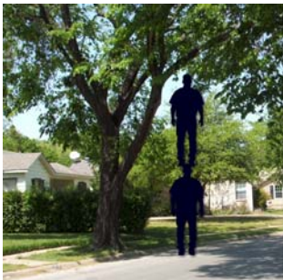
Proper street clearance for trees is more than twice the height of a 6-foot tall person.
