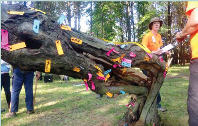
This red maple was pull-tested at Biomechanics Week. First, it failed above the open cavity. Second, a tension root with mower damage broke. It took over 4 tons of pull to separate the woundwood fibers. After the brush was cut off, the trunk was pushed back to vertical. Response growth will be assessed at the next Biomechanics Week.
