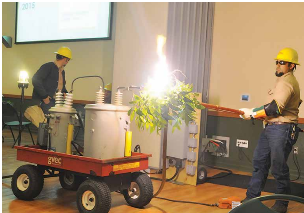
Demonstrating what happens when leaves touch electrical conductors.
