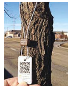
Cable-secured RFID or QR tags are more difficult to remove from trees.
