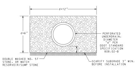
UNDERDRAIN AND BEDDING SECTION
