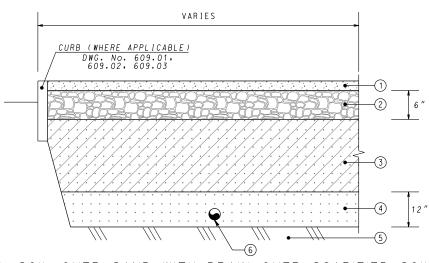
STRUCTURAL SOIL OVER SAND WITH DRAIN OVER SCARIFIED SOIL
