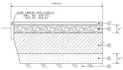
STRUCTURAL SOIL OVER SAND OVER SCARIFIED SOIL
